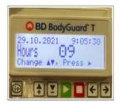
TOGGLE USING THE ARROW BUTTONS TO THE CORRECT HOUR AND SELECT
