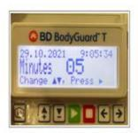
TOGGLE USING THE ARROW BUTTONS TO THE CORRECT MINUTE AND SELECT
